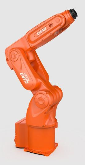
•The overall system architecture of the robot is compact, lightweight, large workspace, fast response, high repeat positioning accuracy, applicable to assembly, sorting, handling, loading and unloading applications.
